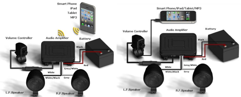
Figure 3. Wiring diagram for Waterproof Bluetooth Audio System. Please note that the wiring plan is the same for both Bluetooth and 3.5mm AUX users.
